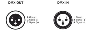
If you are using controllers with this occupation, you can connect the DMX-output of the controller directly with the DMX-input of the first fixture in the DMX-chain. If you wish to connect DMX-controllers with other XLR-outputs, you need to use adapter-cables.
