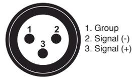
If you are using controllers with this occupation, you can connect the DMX-output of the controller directly with the DMX-input of the first fixture in the DMX-chain. If you wish to connect DMX-controllers with other XLR-outputs, you need to use adapter-cables.
