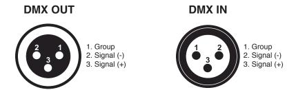
If you are using controllers with this occupation, you can connect the DMX-output of the controller directly with the DMX-input of the first fixture in the DMX-chain. If you wish to connect DMX-controllers with other XLR-outputs, you need to use adapter-cables.
